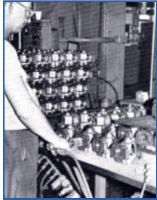
Operator prepares to deburr compressor casting at Copelan Corporation's Sidney, OH facility. The hone is powered by an air tool.
